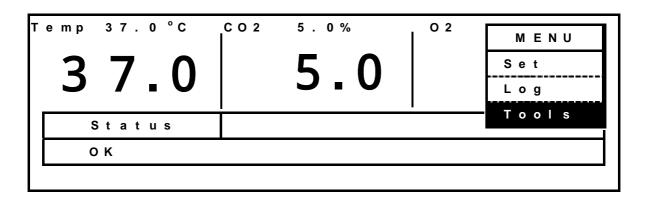
**2.** Select *Key Lock PW Setting* from the Select Tools Display, press the MENU Key to display the menu, select *OK*, and press the ENTER Key.
